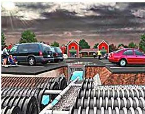
One of the most economical ways to store water underground is in large corrugated high-density polyethylene (HDPE) pipes (see adjacent picture). Strong enough to support the weight of an automobile, these pipes may be discretely buried underneath the parking lot.
