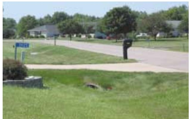
Using roadside swales instead of curbs and gutters helps rainwater infiltrate and reduces the need for storm sewer infrastructure.
